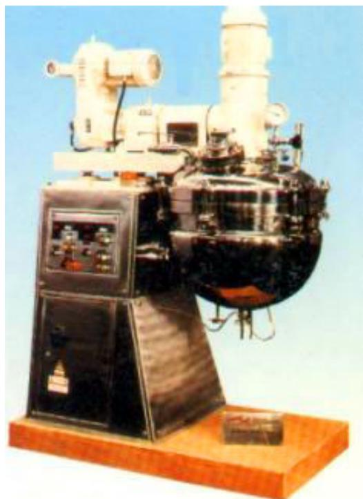
**Figure 9.9: b) Small desktop model of a vacuum mixer.**
